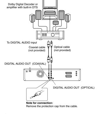
Connect the unit and a Dolby Digital decoder or an amplifier with built-in DTS using either an optional optical cable or an optional coaxial cable.
